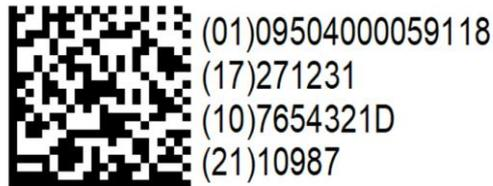
**Figure 5-2** Example of a GS1 DataMatrix
