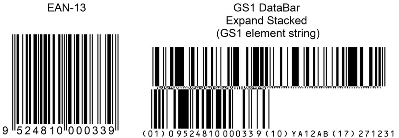
**Figure 4-1** Example of POS linear barcodes
