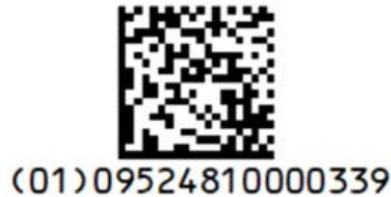
**Figure 7-2** Example of retail POS GS1 DataMatrix
