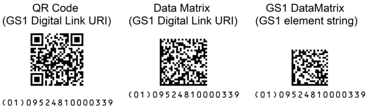
**Figure 4-2** Example of POS 2D barcodes
