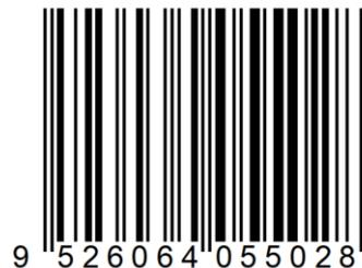
**Figure 5-1** Example in an EAN-13
