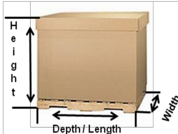
Figure 5-8 Dimensions of bulk loads on shipping platforms
