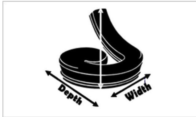
Figure 4-78 Curved stairway component measurement
