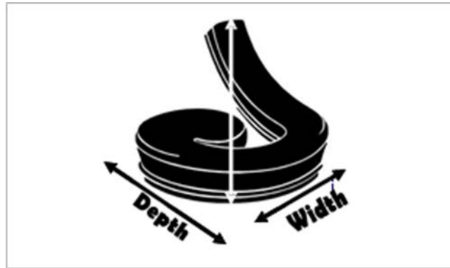
Figure 4-78 Curved stairway component measurement
