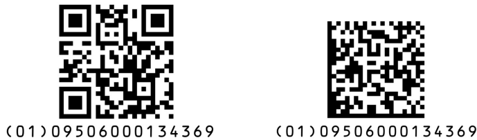
Figure 2-32-3 Examples of QR Code and Data Matrix with GS1 DL URI Syntax
