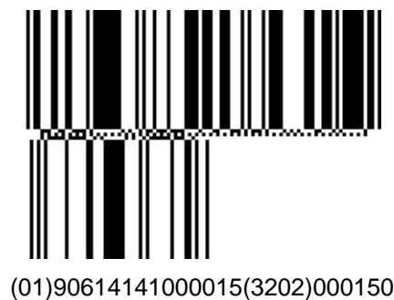
Figure A1.3 - 1 Example of GS1 DataBar Expanded Stacked Bar Code Symbol that uses concatenation
