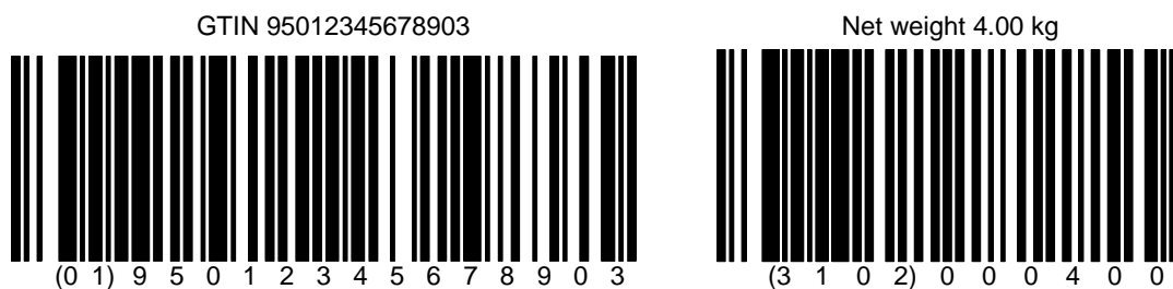
Figure A.1.1 – 1 Data Encoded in two GS1-128 symbols
