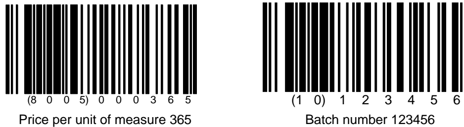
Figure A1.2 – 1 Data Encoded in two GS1-128 symbols
