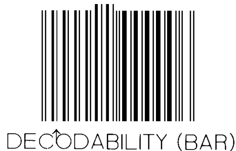
Figure 5.5.3.3.12 - 3 Calibration Symbol with Engineered Low Decodability Grade
