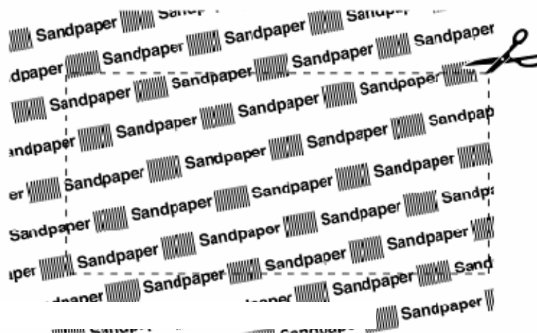
Figure 6.3.3.7 - 2 Bar Code Symbol Placement on Random-Wrapped Item
