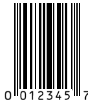
Figure 5.2.2.3.4 - 1 UPC-E Bar Code Symbol (Encoding 00123400057 by Zero-Suppression)
