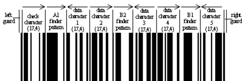
Figure 5.5.2.4 – 1: RSS Expanded Structure
