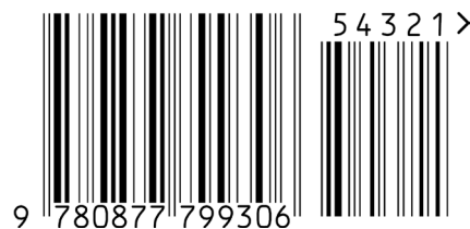
Figure 5.2.1.3.5.2-2. EAN-13 barcode with five-digit add-on symbol
