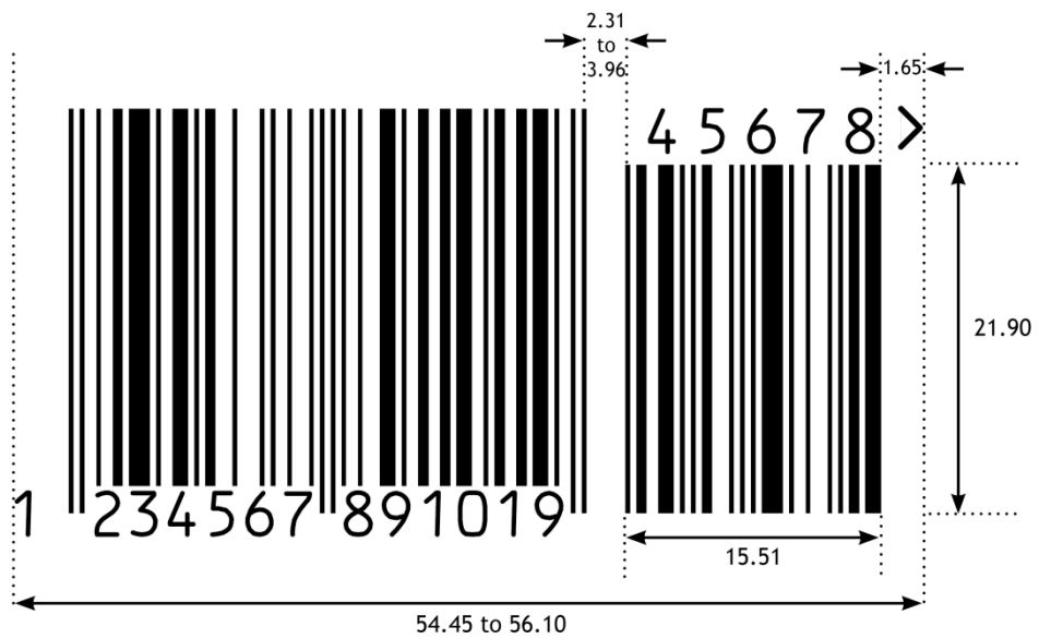
Figure 5.2.4.6-6. EAN-13 barcode with five-digit add-on symbol
