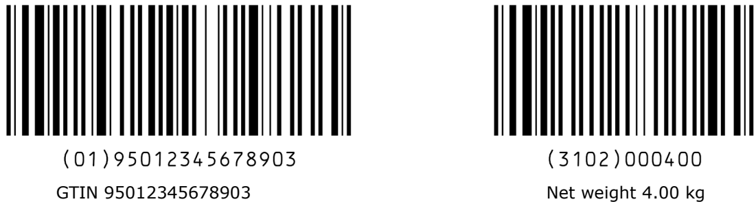
Figure 5.10.2.1-2. Data encoded in one concatenated GS1-128 symbol
