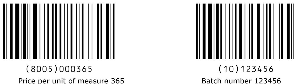
Figure 5.10.2.2-1. Data encoded in two GS1-128 symbols
