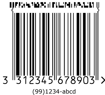
Figure 5.8.8-1. EAN-13 symbol with a four-column CC-A component
