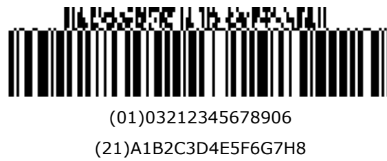
Figure 5.8.8-9. GS1-128 symbol with a four-column CC-A
