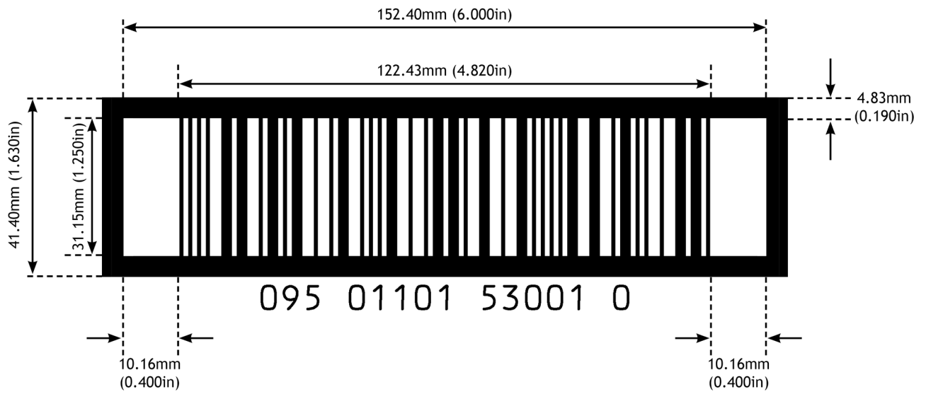
Figure 5.3.6-1. ITF-14 symbol: Main dimensions at X-dimension 1.016 mm (0.0400 in.)
