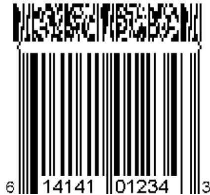
Figure 5.8.8-2. UPC-A symbol with a four-column CC-B component
