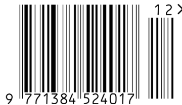
Figure 5.2.1.3.5.1-2. EAN-13 barcode with two-digit add-on symbol
