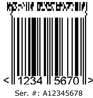
Figure 5.8.8-3. EAN-8 symbol with a three-column CC-A
