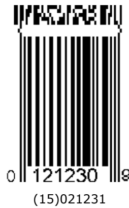
Figure 5.8.8-4. UPC-E symbol with a two-column CC-A
