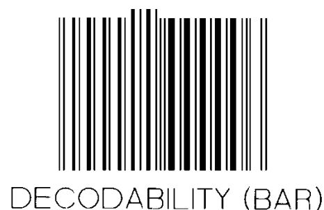
Figure 5.5.3.3.12-3. Calibration symbol with engineered low decodability grade
