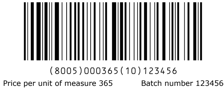
Figure 5.10.2.2-2. Data encoded in one concatenated GS1-128 symbol
