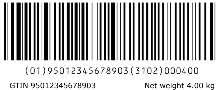
Figure 5.10.2.1-2. Data encoded in one concatenated GS1-128 symbol
