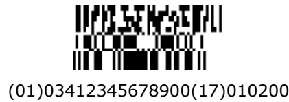
Figure 5.8.8-6. GS1 DataBar Stacked symbol with a two-column CC-A
