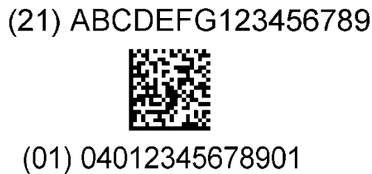
Figure 2.1.4-4. Example of GS1 DataMatrix symbol encoded with GTIN and serial number AI (21)
