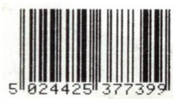
Figure 5.5.3.3.12-1. Symbol with Edge Determination Problem
