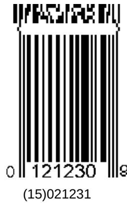
Figure 5.10.2.3-2. Example of mixed GS1 Symbolologies (GTIN encoded in UPC-E, Best Before Date in Composite)
