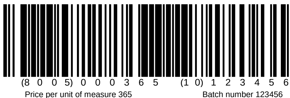
Figure 5.10.2.2-2. Data Encoded in one Concatenated GS1-128 symbol
