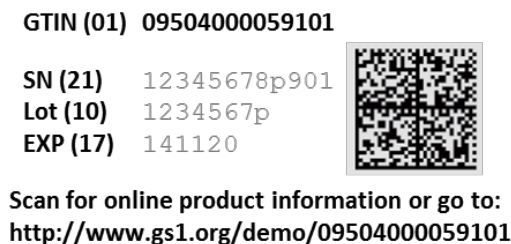
Figure 4.14.1-2. Combination of HRI with AIs, Non-HRI Text and data titles
