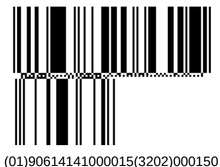
Figure 5.10.2.3-1. Example of GS1 DataBar Expanded Stacked Barcode that uses concatenation
