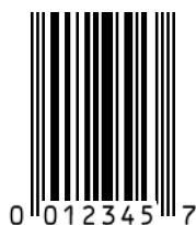
Figure 5.2.1.3.4-1. UPC-E Barcode (Encoding 001234000057 by Zero-Suppression)
