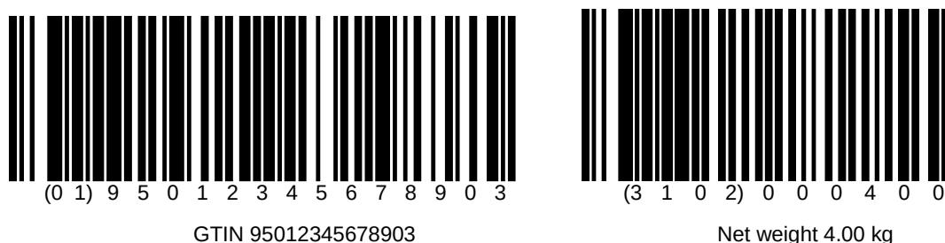
Figure 5.10.2.1-1. Data Encoded in two GS1-128 symbols
