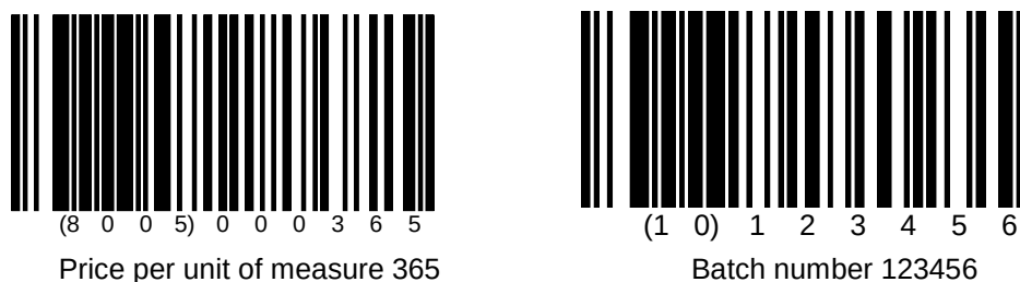
Figure 5.10.2.2-1. Data Encoded in two GS1-128 symbols
