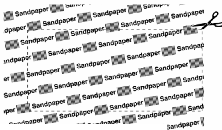
Figure 6.3.3.7 – 2. Bar code placement on random-wrapped item
