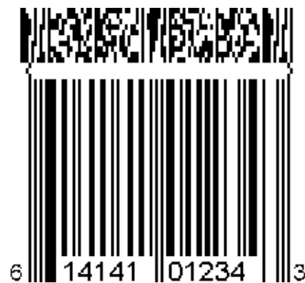
Figure 5.8.8 – 2. UPC-A Symbol with a Four-Column CC-B Component
