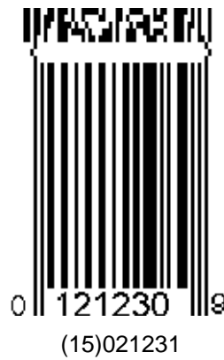
Figure 5.8.8 – 4. UPC-E Symbol with a Two-Column CC-A
