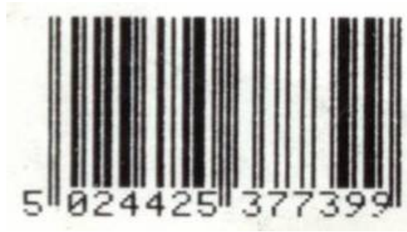
Figure 5.5.3.3.12 – 1. Symbol with Edge Determination Problem
