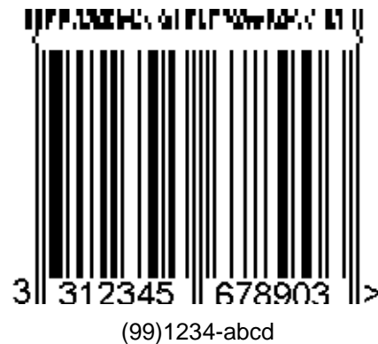
Figure 5.8.8 – 1. EAN-13 Symbol with a Four-Column CC-A Component
