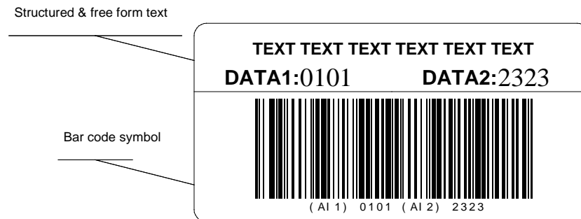
Figure 6.7.3.2 – 1. Bar code and Human Readable Interpretation Layout
