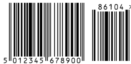
Figure 5.2.1.3.5.2 – 2. EAN-13 Bar Code with Five-Digit Add-On Symbol
