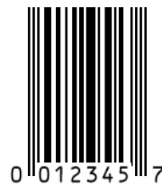
Figure 5.2.1.3.4 – 1. UPC-E Bar Code (Encoding 001234000057 by Zero-Suppression)
