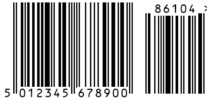
Figure 5.2.1.3.5.2 – 2 EAN-13 Bar Code with Five-Digit Add-On Symbol
