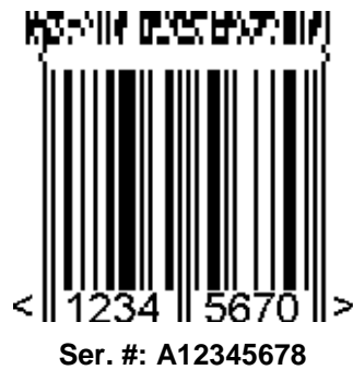
Figure 5.8.8 - 3 EAN-8 Symbol with a Three-Column CC-A
