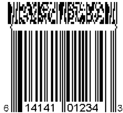
Figure 5.8.8 - 3 EAN-8 Symbol with a Three-Column CC-A
