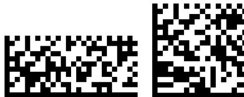
Figure 5.7.3.1 - 1 Rectangular and Square GS1 DataMatrix Symbols
