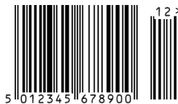
Figure 5.2.1.3.5.1 - 2 EAN-13 Bar Code with Two-Digit Add-On Symbol
