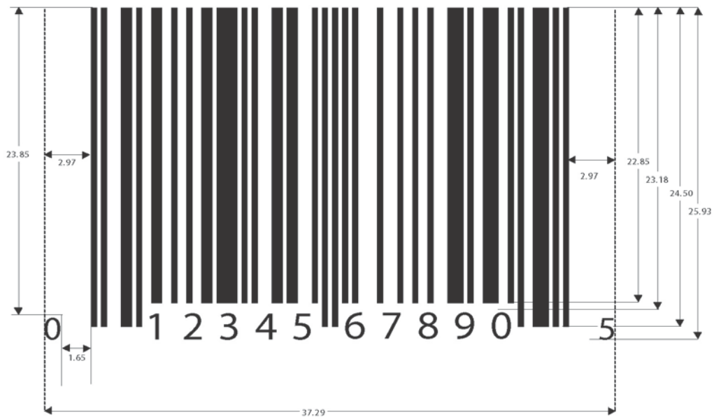
Figure 5.2.3.6 - 2 UPC-A Bar Code
