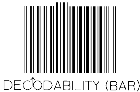
Figure 5.5.3.3.12 - 3 Calibration Symbol with Engineered Low Decodability Grade
