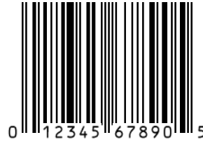
Figure 5.2.1.3.3 - 1 UPC-A Bar Code
