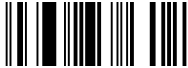
Figure 5.1 - 4 GS1 DataBar Omnidirectional Bar Code
