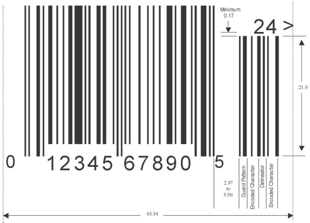
Figure 5.2.3.6 - 6 UPC-A Bar Code with Two-Digit Add-On Symbol
