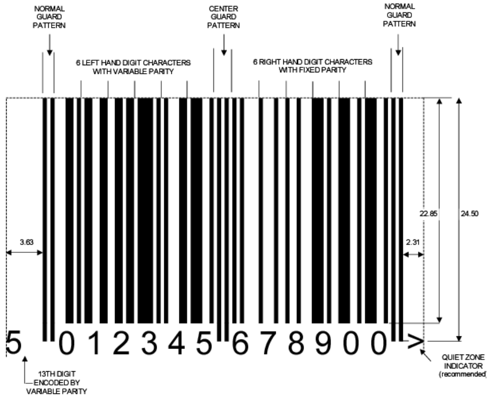
Figure 5.2.3.6 - 2 UPC-A Bar Code
