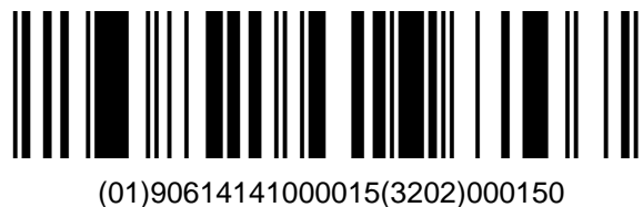
Figure 5.6.1.4.1 - 1 GS1 DataBar Expanded Bar Code
