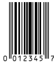
Figure 5.2.1.3.4 - 1 UPC-E Bar Code (Encoding 001234000057 by Zero-Suppression)
