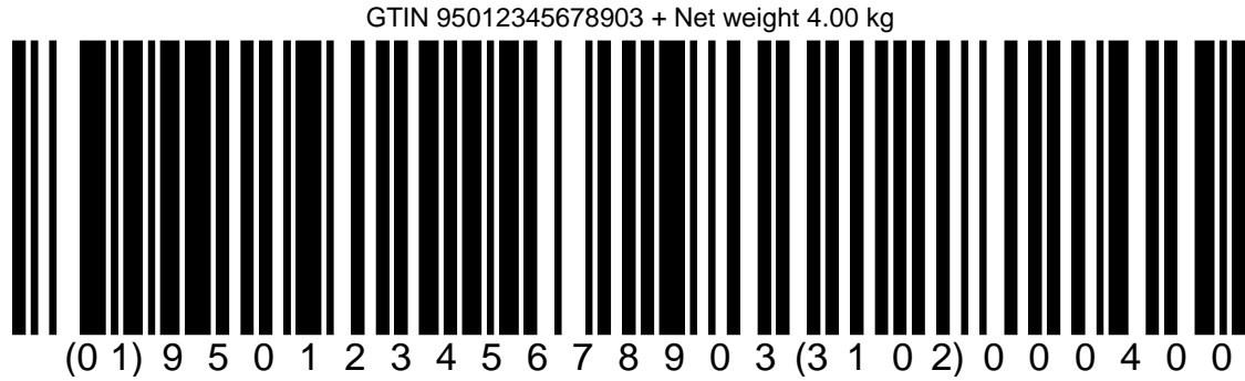
Figure A.1.1 – 2 Data Encoded in one Concatenated GS1-128 symbol
