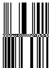
Figure 5.6.1.2.4 - 1 GS1 DataBar Stacked Omnidirectional Bar Code
