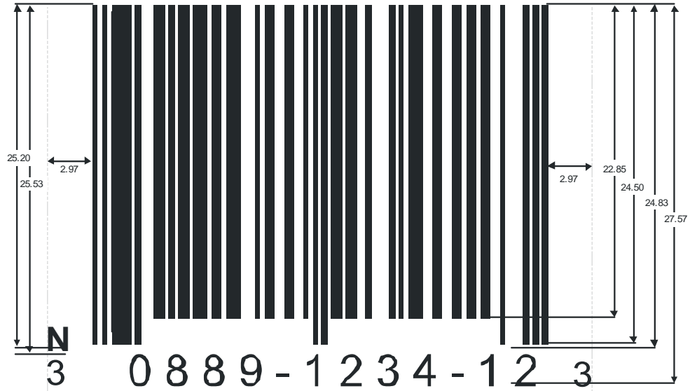
Figure 5.2.3.6 - 3 UPC-A Bar Code
