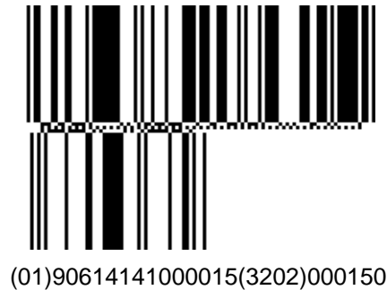
Figure A1.3 - 1 Example of GS1 DataBar Expanded Stacked Bar Code that uses concatenation
