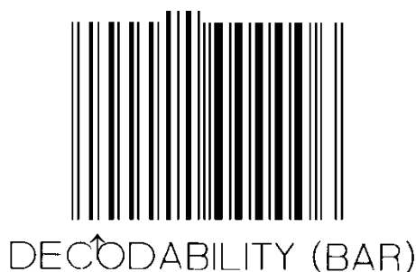
Figure 5.5.3.3.12 - 3 Calibration Symbol with Engineered Low Decodability Grade
