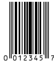
Figure 5.2.2.3.4 - 1 UPC-E Bar Code (Encoding 001234000057 by Zero-Suppression)
