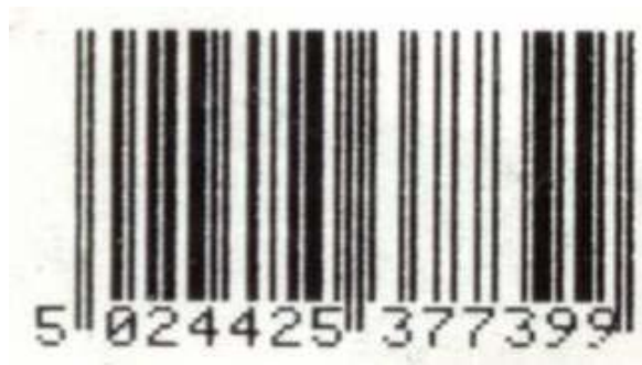
Figure 5.5.3.3.12 - 1 Symbol with Edge Determination Problem
