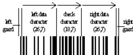
Figure 5.6.1.3 - 2 GS1 DataBar Limited Bar Code Structure
