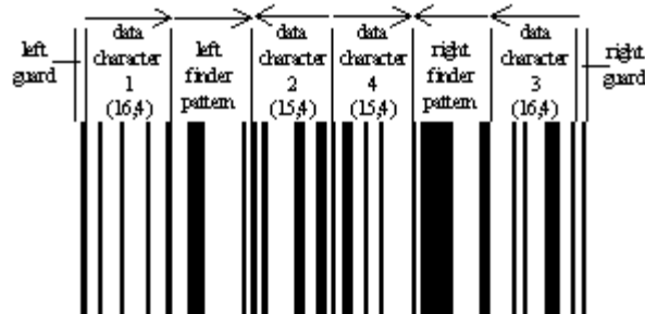
Figure 5.6.1.2 - 1 First Group of GS1 DataBar Symbols Structure
