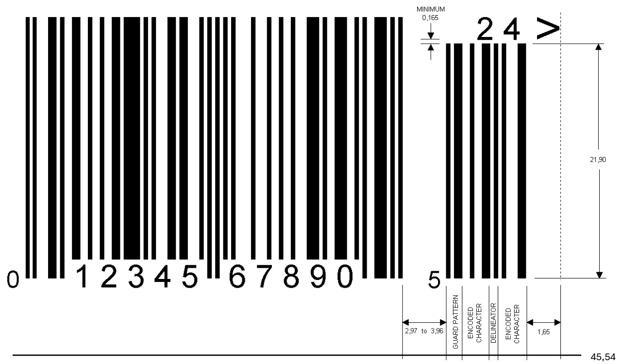
Figure 6: UPC-A with 2-digit add-on
