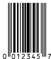
Figure 4: UPC-E bar code symbol (encoding “00123400057” by zero suppression)
