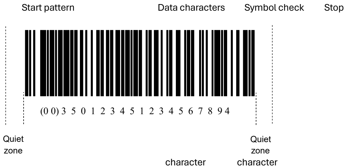
Figure 1: General format of UCC/EAN-128 symbol
