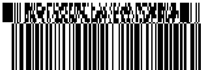
Figure 5.11.2-2. GS1-128 Composite symbol with CC-C
