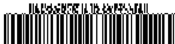
Figure 5.11.8-9. GS1-128 symbol with a four-column CC-A
