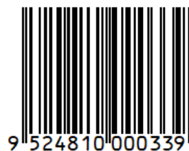
Figure 4.14-5. Example of EAN-13 with EAN/UPC HRI format
