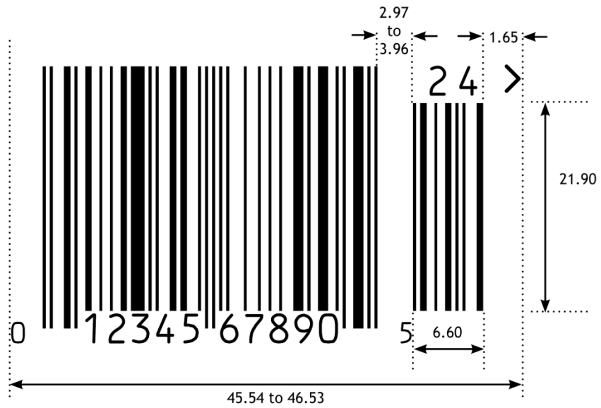
Figure 5.2.6.6-5. UPC-A barcode with two-digit add-on symbol
