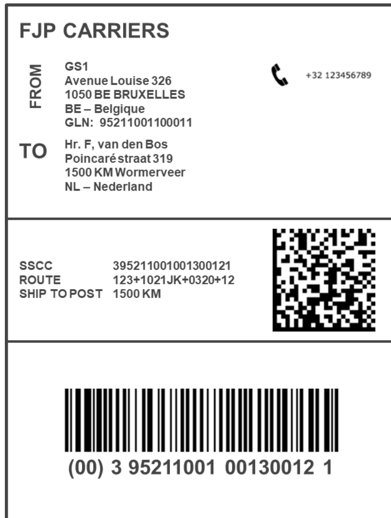
Figure 6.6.5-8 Label GS1 DataMatrix encoding transport process information
