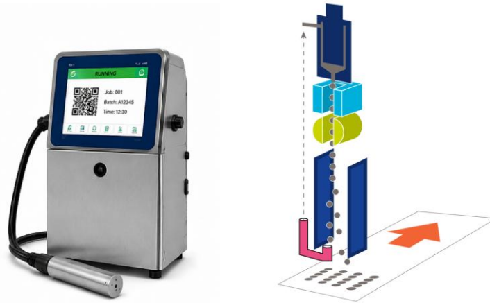
Figure 6-1 Example of CIJ printer and printing method
