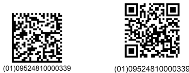
Figure 4-5 Example of Data Matrix (left) and QR Code (right)
