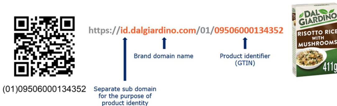
Figure 4-6 Example of a QR Code with GS1 Digital Link URI syntax
