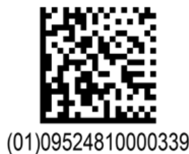
Figure 4-3 Example of a retail GS1 DataMatrix
