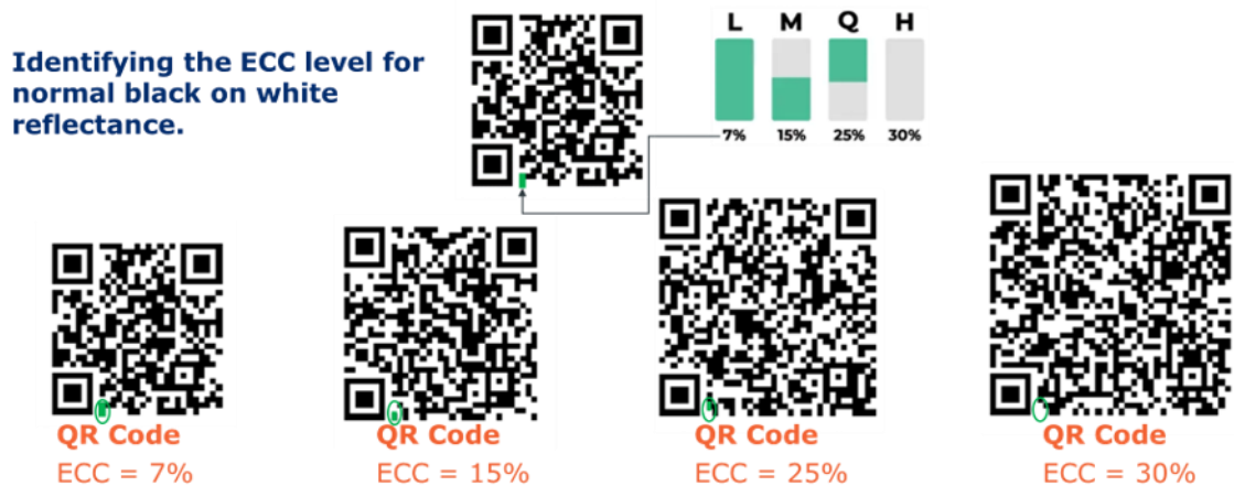
Figure 5-3 Example of ECC level indicator
