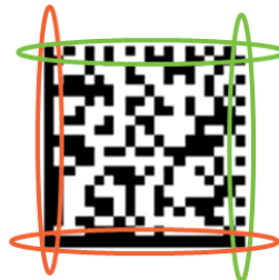
Figure 5-1 Example of the Data Matrix finder pattern
