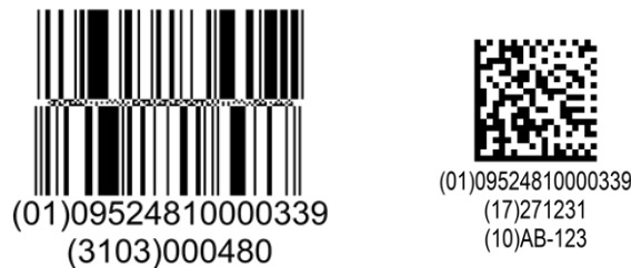
Figure 4-2 Example of GS1 DataBar Expanded Stack (left) and GS1 DataMatrix (right)
