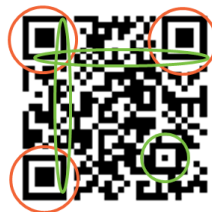
Figure 5-2 Example of the QR Code finder pattern
