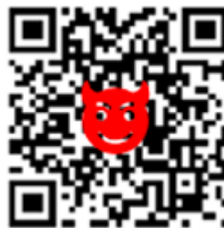
Figure 5-16 An example using a logo within a QR Code with ECC (M) error correction results in a failure
