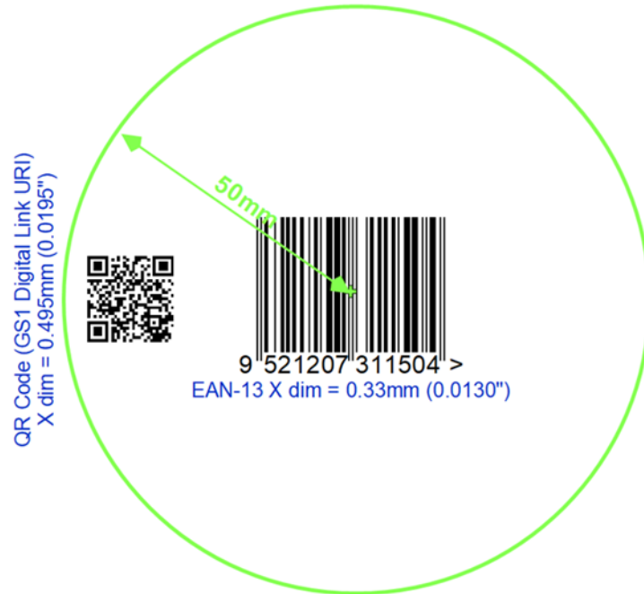
Figure 5-11 2D barcode placement in relation to the linear barcode for POS
