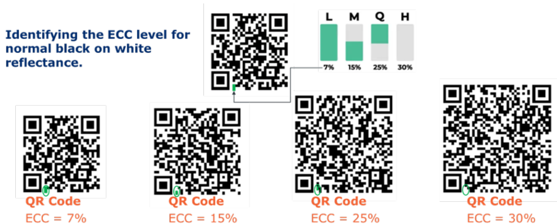
Figure 5-3 Example of ECC level indicator
