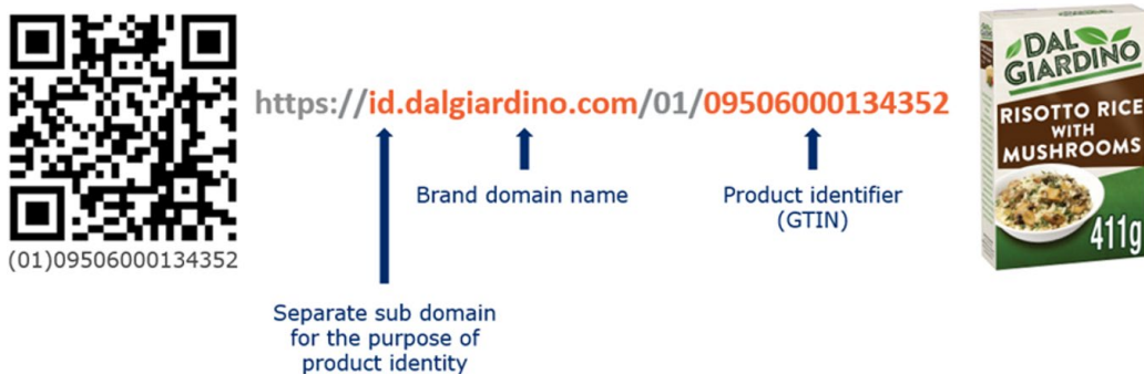
Figure 4-6 Example of a QR Code with GS1 Digital Link URI syntax
