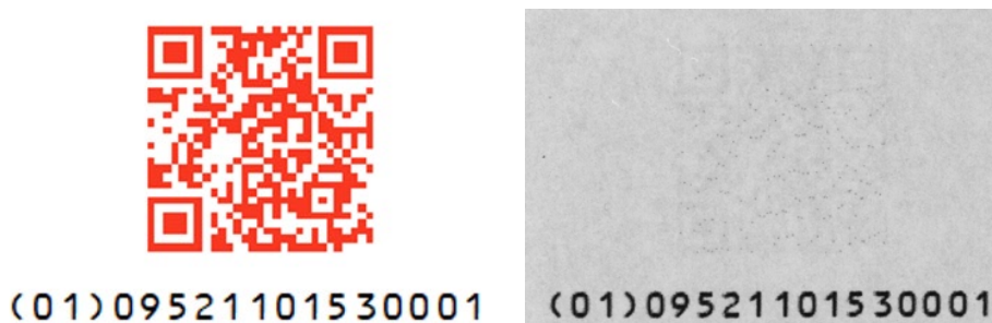
Figure 5-15 View of red QR Code by a smart device imager (left) and a red illuminated POS imager (right)
