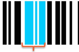
Enlarged section of first part of a GS1-128 barcode showing the Function 1 character in blue
