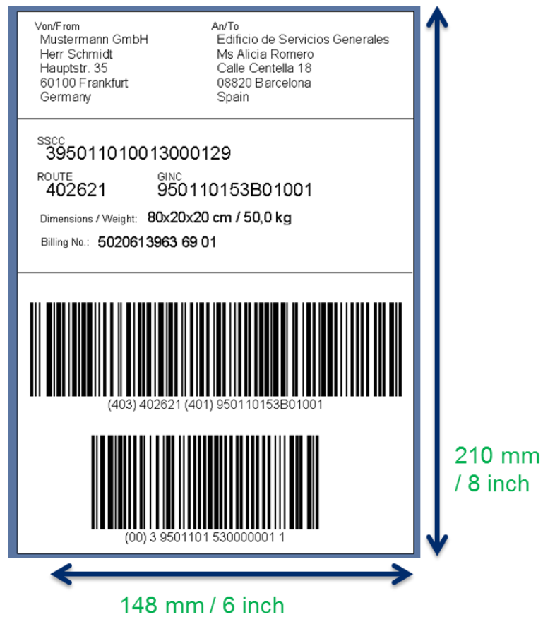
Figure 7-2 dimensions of A5 / 6 x 8 inch label
