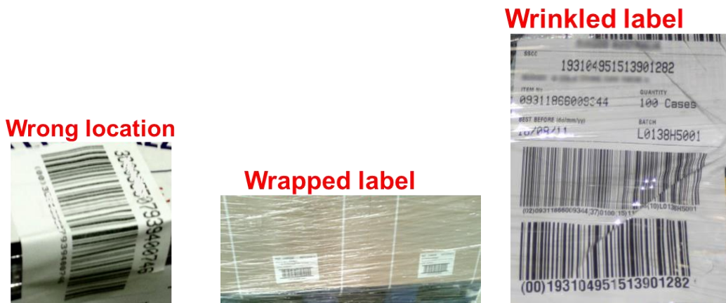
Figure 9-3 Examples of placement issues
