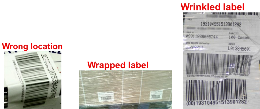
Figure 9-3 Examples of placement issues
