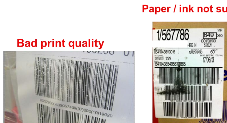
Figure 9-2 Examples of printing-related problems
