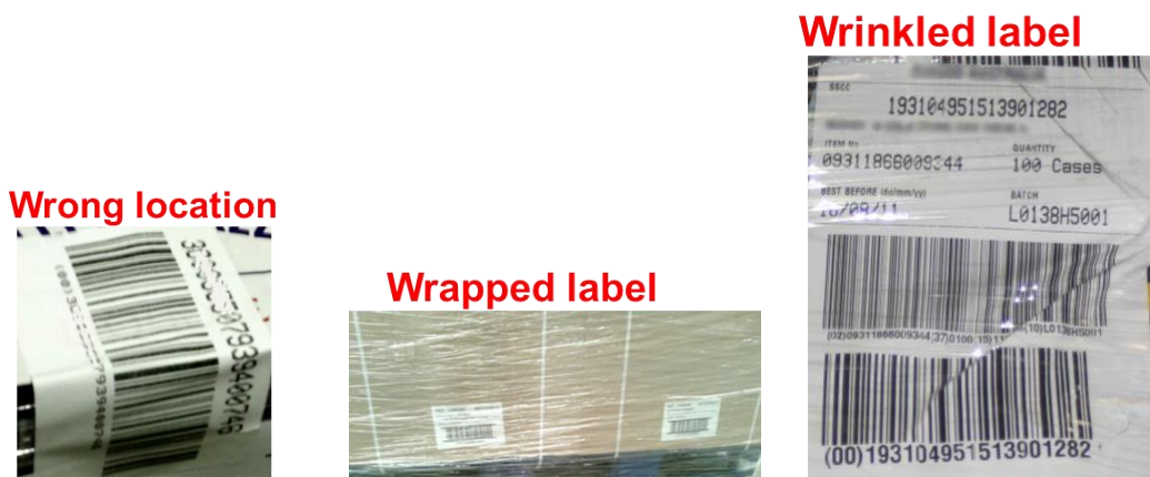
Figure 9-3 Examples of placement problems
