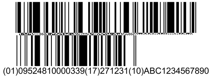
Figure 3-15 Example of correct HRI, all AIs and their corresponding values are placed on the same line
