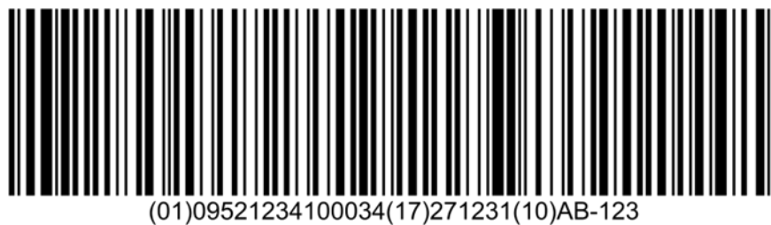
Figure 3-4 Example of a GS1-128 with multiple GS1 element strings, HRI is grouped together and placed below the barcode
