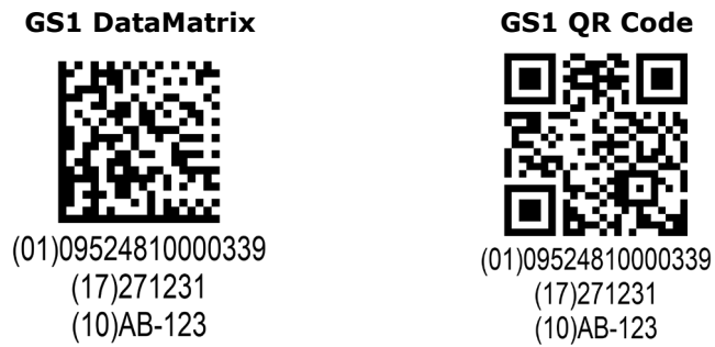
Figure 3-6 Examples the HRI grouped together under the barcodes
