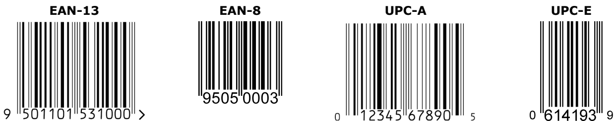
Figure 3-1 Some correct examples of EAN/UPC barcodes, the HRI is placed at the bottom
