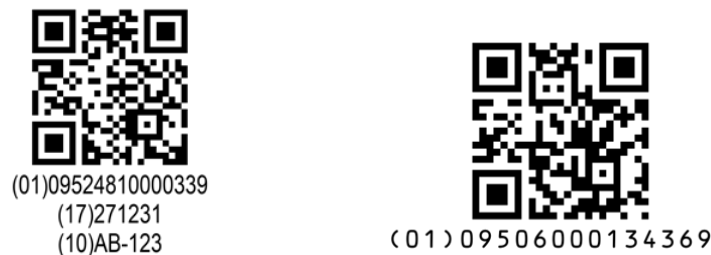
Figure 2-6 Examples of GS1 QR Code (left) and QR Code (right) barcodes
