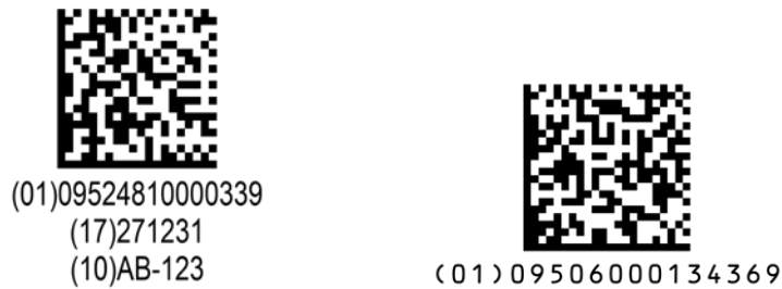
Figure 2-5 Examples of GS1 DataMatrix (left) and Data Matrix (right) barcodes
