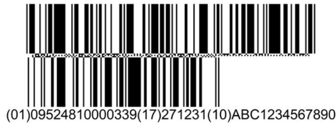
Figure 3-22 Example of parentheses around AIs
