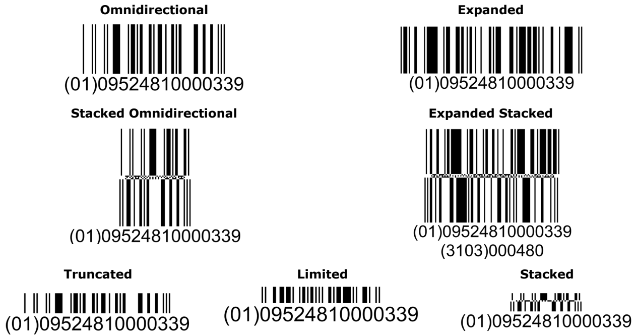
Figure 2-4 Example of GS1 DataBar barcodes
