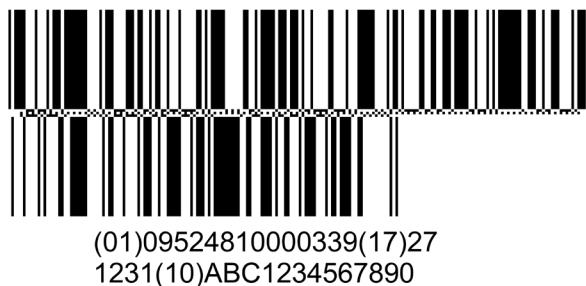
Figure 3-17 Example of HRI improperly split across multiple
