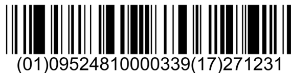
Figure 3-5 Example, HRI grouped together and placed below the GS1 DataBar Expanded barcode:
