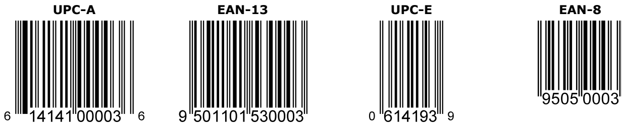
Figure 2-1 Examples of EAN/UPC barcodes
