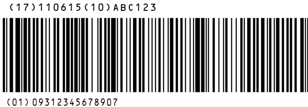
Figure 3-19 Example the HRI of the above and below GS1-128 barcode
