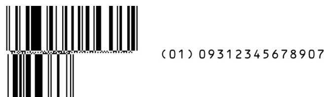
Figure 3-13 Example of a GS1 DataBar Expanded Stacked barcode with HRI placed to the right barcode
