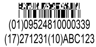
Figure 2-7 Example of GS1 Composite barcode.
