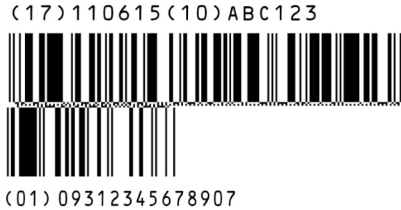
Figure 3-18 Example the HRI of the above and below GS1 DataBar barcode
