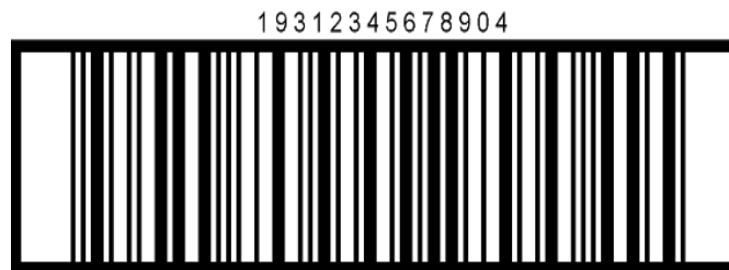
Figure 3-12 Example, the HRI is placed above the ITF-14 barcode
