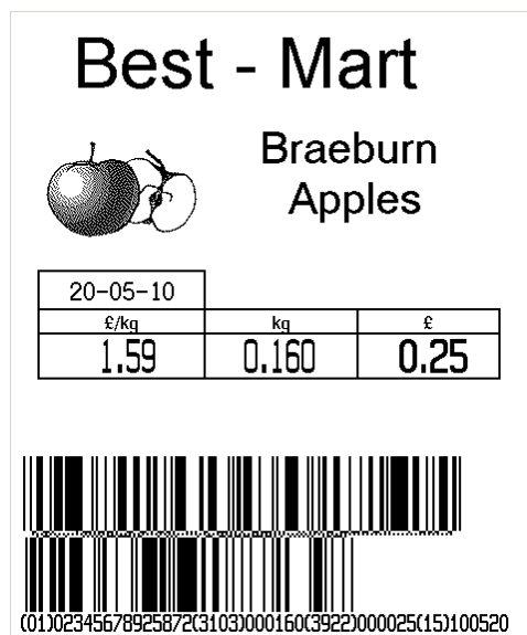
Figure 4-2 To-Be label using a GS1 DataBar Expanded Stacked encoding GTIN plus additional data
