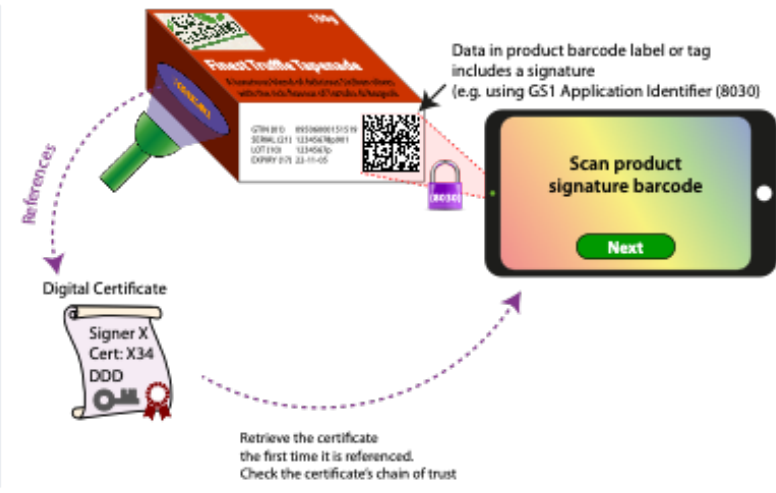
Figure 3-2 Example of DigSig AI (8030) encoded as GS1 element string in a 2D barcode
