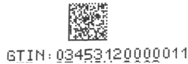
Figure 4-1 Inkjet printed GS1 DataMatrix
