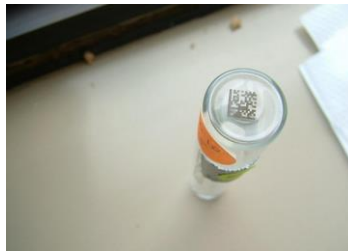
Figure 4-2 GS1 DataMatrix Laser symbol
