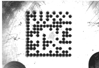
Figure 4-3 GS1 DataMatrix dot-peen symbol
