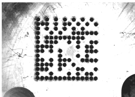
Figure 4-3 GS1 DataMatrix dot-peen symbol
