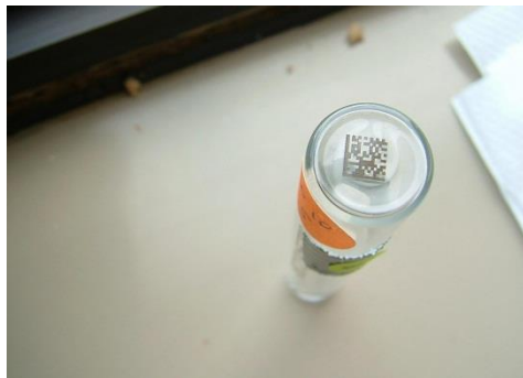
Figure 4-2 GS1 DataMatrix Laser symbol
