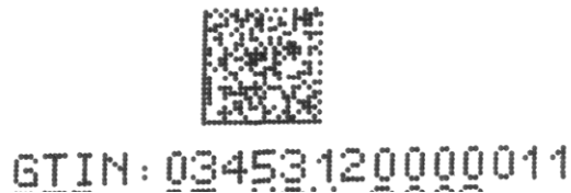
Figure 4-1 Inkjet printed GS1 DataMatrix
