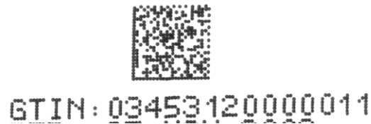
Figure 4-1 Inkjet printed GS1 DataMatrix
