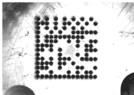
Figure 4-3 GS1 DataMatrix dot-peen symbol
