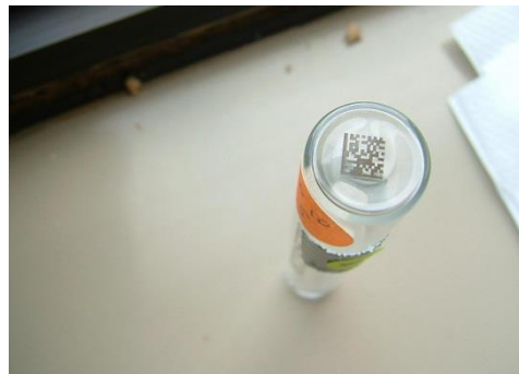
Figure 4-2 GS1 DataMatrix Laser symbol
