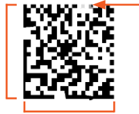
Figure 4.6.1.2-5 Fixed Pattern Damage
