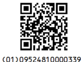
Figure 5-1 Example of QR Code with GS1 Digital Link URI data string: https://example.com/01/09524810000339/10/YA12AB?17=271231
