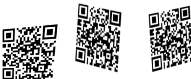
Figure 7-8 Examples of grid non-uniformity
