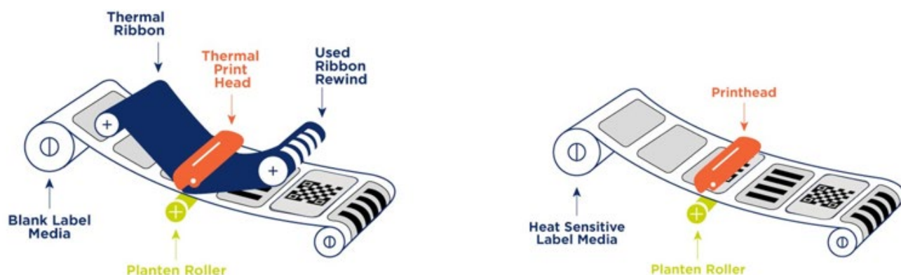
Figure 8-9 Example of thermal transfer and direct thermal label printing
