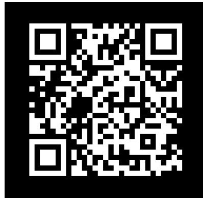
Figure 2-4 QR Code Quiet Zone reverse reflectance example
