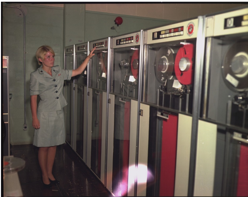
PFC Patricia Barbeau operates a tape-drive on the IBM 729 at Camp Smith, Hawaii, October 1969
