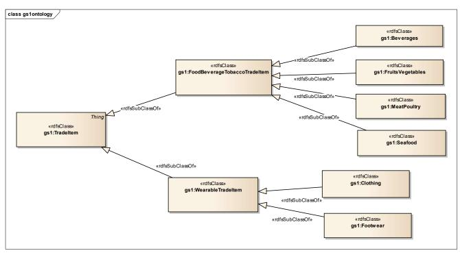
Note: The associations in the above class diagram describe inheritance between classes. A subclass is derived from a parent class.
